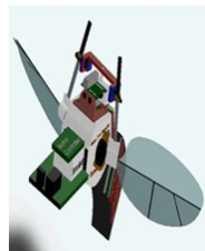
(a) The CAE SolidWorks model of the recently designed Bumblebee MAV prototype.
